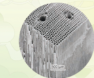
クロマツ木口面（横断面）の走査電子顕微鏡写真 Scanning electron microscope image of the cross-section of a black pine trunk
